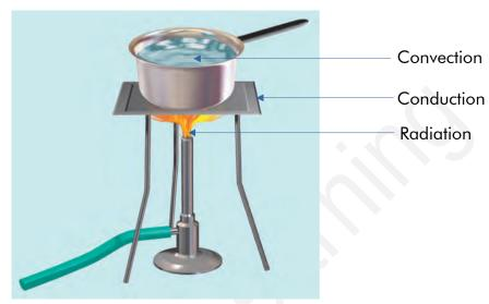
Conduction: Heat transfer from the flame to the pan through the metal base.
