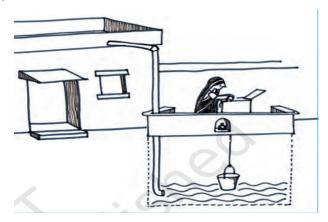
**Ans**. The water collected on the roof comes down in the pipes and gets stored in the tank below.
